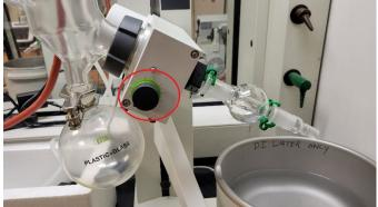
• Lower the flask into the water bath using the front handle. Squeeze the handle to release the catch.
