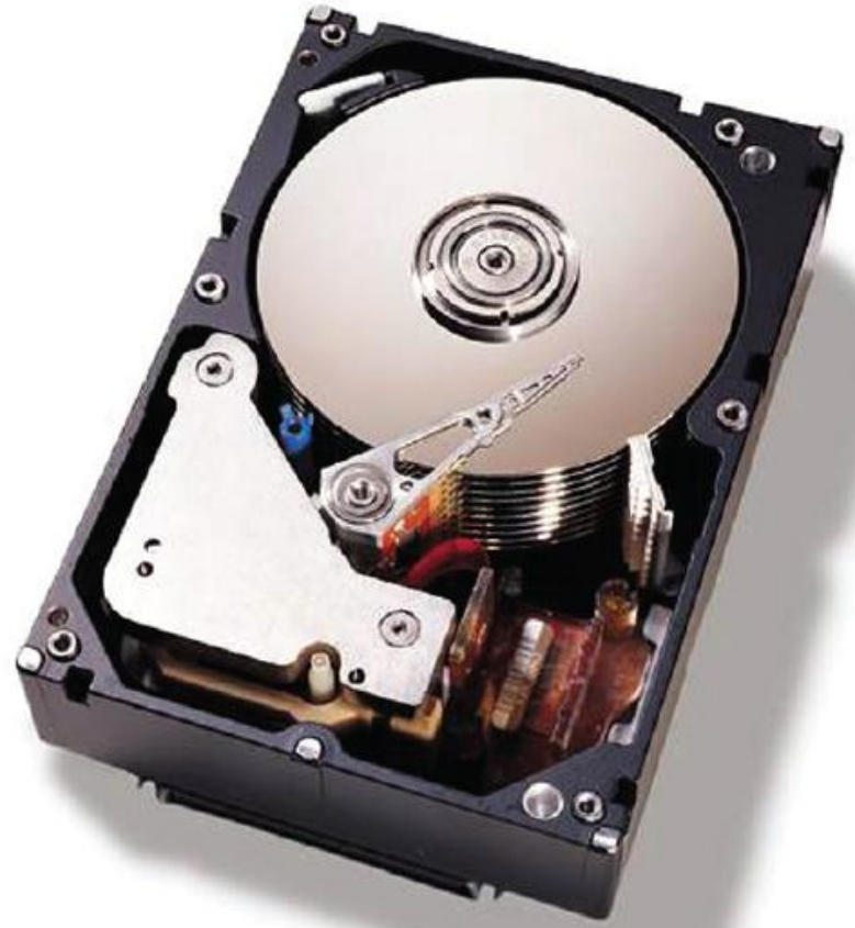
Figure 1.11 Top view of a 36 GB, 10,000 RPM, IBM SCSI server hard disk, with its top cover removed. Note the height of the drive and the 10 stacked platters. (The IBM Ultrastar 36ZX.)
